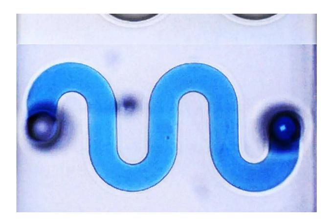
A 3D printed glass microfluidic channel, shown hollow and filled with liquid. Credit: Georgia Institute of Technology
