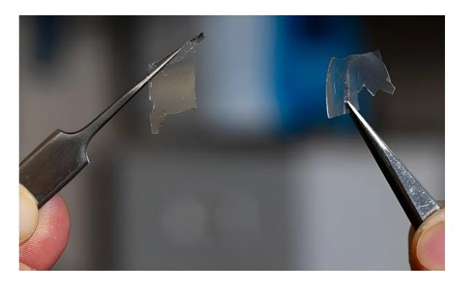
Researchers used this raw material to create 3D-printed glass structures no bigger than the width of a human hair. The researchers employed a lightsensitive resin based on a widely used soft polymer called PDMS, at left. The sample on the right is glass created using deep UV light to convert the the photoresin to hardened inorganic glass. Credit: Candler Hobbs
