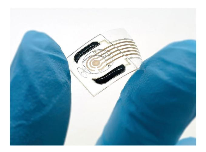
A wireless sweat sensor developed in the lab of Caltech's Wei Gao monitors levels of estradiol, an important female hormone that plays a role in health and fertility. Credit: Caltech
