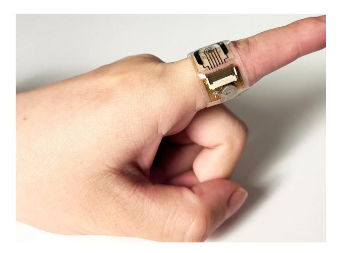
The sensor, as worn around the index finger. Credit: Caltech
