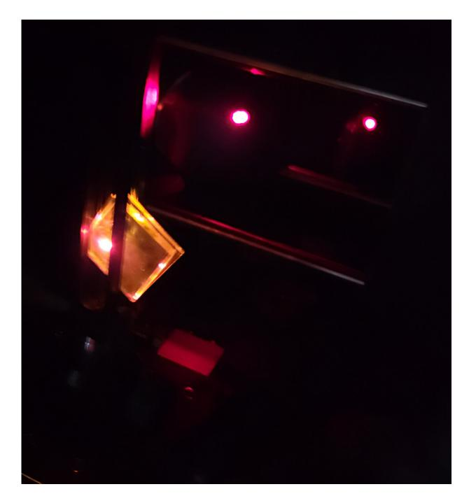
The thin film with emitter solution added and encapsulated upconverts lower energy red light to higher energy yellow light. Credit: Exciton Science
