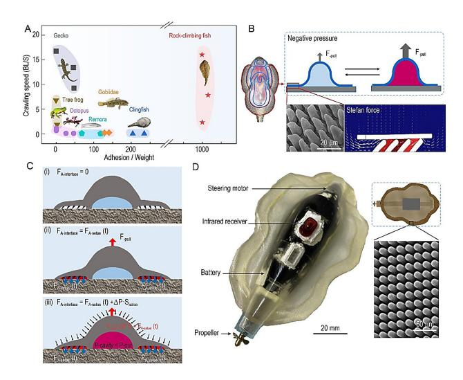
(A) Among the adhering species, the rock-climbing fish can generate great adhesion force with amazing crawling ability underwater. (B) The setae array on the brown shaded area conforms to the substrate and forms a sealing chamber through the Stefan force; the inner cavity of the suction cup in the blue area
