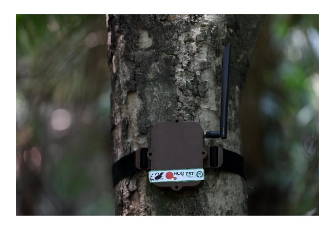
The 'curupira' sensors look like small internet modems but are in fact wireless and can relay data up to one kilometer (0.6 miles) via satellite to others in a network.
