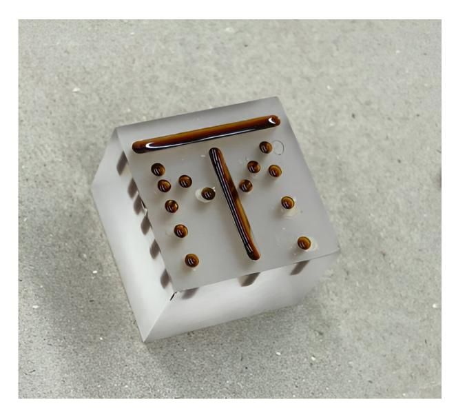
Closeup of the quartz glass cube that holds the magnetic nanoparticles in solution. The brown liquid is the solution of nanoparticles. Credit: Thinh Bui/NIST
