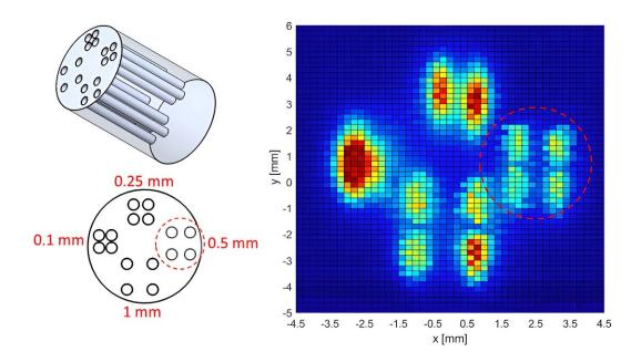
Left: Diagram of the series of tiny wells, in clusters of fours, filled with solution. Each well in a foursome is spaced away from the other wells by a certain amount, anywhere from 0.1 mm (very close together) to 1 mm (further apart). Right: The magnetic particle image itself, showing distinctions between the wells spaced farther apart but not between the wells spaced close together. The dashed red circle in both images shows the foursome of wells spaced 0.5 mm apart. Credit: NIST
