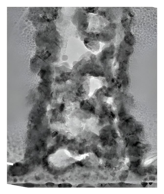
The irregular interior structure of a nanoscale nickel pillar. Credit: Caltech
