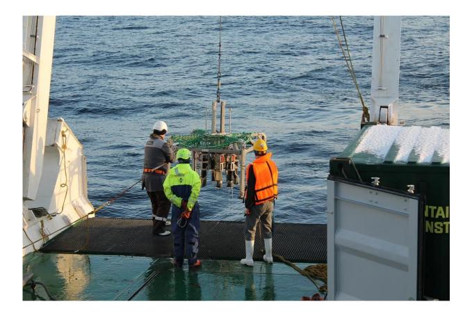
Extraction of bottom multicorer sampler with bottom water and sediments. Credit: Members of the AMK-82 Arctic expedition in 2020
