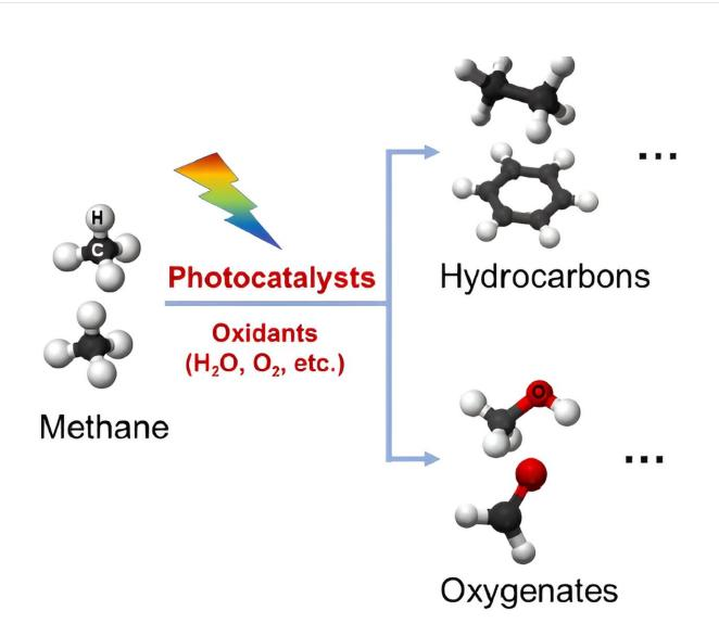
Photocatalysis uses sunlight or artificial light sources as the only energy input to selectively oxidize methane to C2+ hydrocarbons or oxygenates using low-cost, environmentally friendly oxidants, such as water and oxygen at low temperatures. Credit: Carbon Future, Tsinghua University Press
