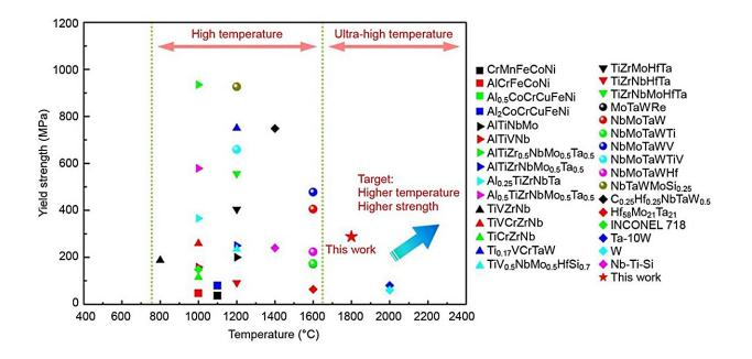
A new type of alloy called the ultra-high-temperature HEA (UHT-HEA) has been proposed, which can serve at temperatures greater than 1800 °C. The NbMoTaWHfN RHEA is reported to exhibit a novel compressed yield strength of 288 MPa at 1800 °C? whereas the highest testing temperature of most alloys is no more than 1600 °C. Credit: Yixing Wan
