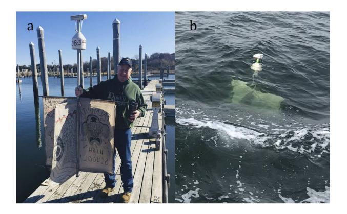
Davis-style surface drifter used to track currents in Cape Cod Bay, Massachusetts. (A) Drifter before deployment to show size comparison. (B) Deployed surface drifter shows main body submerged. Credit: Chip Carroll (A) and Felicia Page (B).
