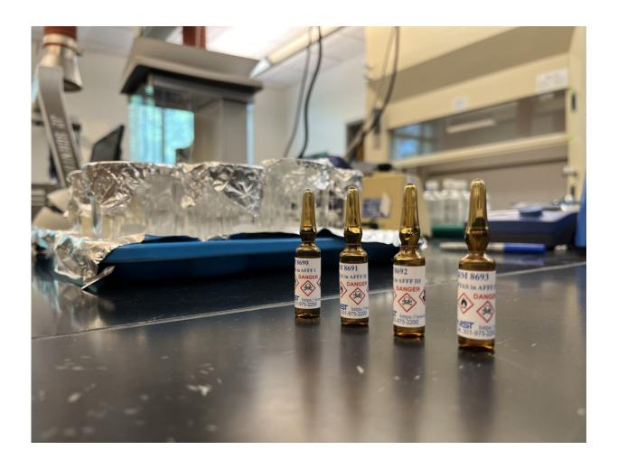
A series of reference materials contains precise measurements of per- and polyfluoroalkyl substances (PFAS), known as forever chemicals, in firefighting foams. These foams, called aqueous film-forming foams (AFFFs), are used to suppress fuel fires. Analytical labs can use the reference materials for measuring
