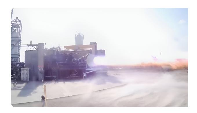
A Raptor Vacuum engine was successfully cold-started during a test in August 2023. Credit: SpaceX
