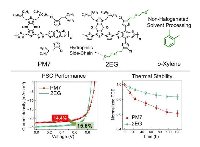
A blend of hydrocarbon and hydrophilic oligoethylene glycol (2EG) performed better than the standard solvent when used in PSC creation, based on overall performance and thermal stability. Credit: Nano Research Energy, Tsinghua University Press
