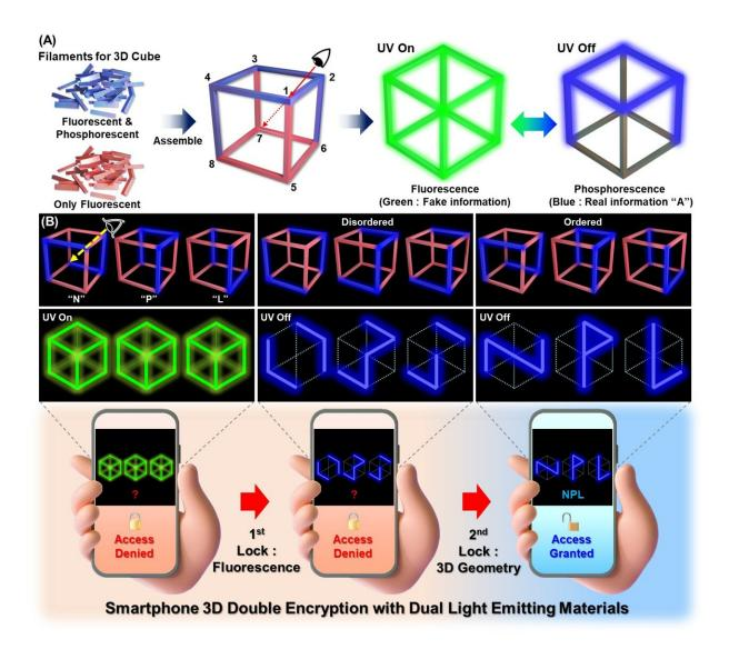
(A) Fabrication process and optical encryption concept of fluorescence and phosphorescence dual-light-emitting 3D cubes. (B) Smartphone based double encryption with 3D dual-light-emitting 3D cubes. Credit: Jin Woo Oh, Seokyeong Lee, Hyowon Han, Omar Allam, Ji Il Choi, Hyeokjung Lee, Wei Jiang, Jihye Jang, Gwanho Kim, Seungsoo Mun, Kyuho Lee, Yeonji Kim, Jong Woong Park, Seonju Lee, Seung Soon Jang, and Cheolmin Park
