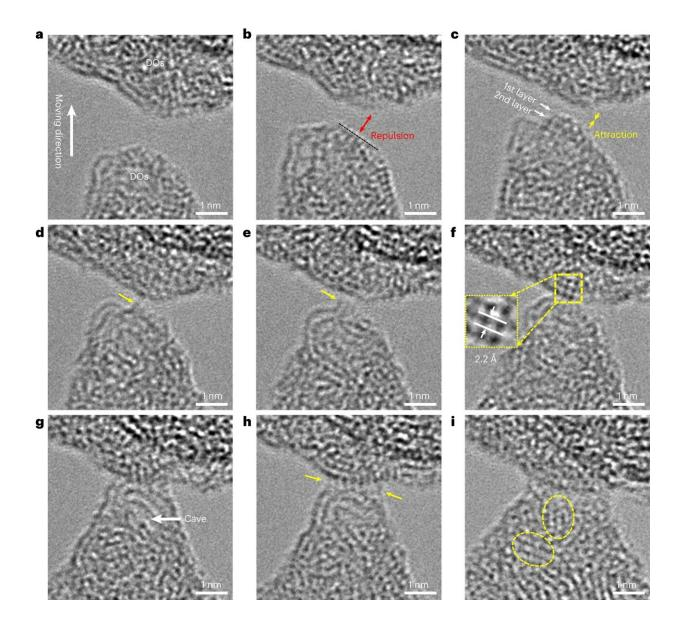
Dynamic healing process of two fractured surfaces with DO protrusions. a-c,
