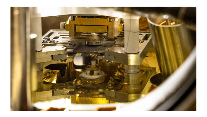
Using the ultrahigh-vacuum atomic force microscope at DOE's Center for Nanophase Materials Sciences at ORNL, researchers found unique environmentally induced ferroelectric phase transitions in hafnium zirconium oxide, a material important in developing advanced semiconductors. Credit: Arthur Baddorf/ORNL, Dept. of Energy
