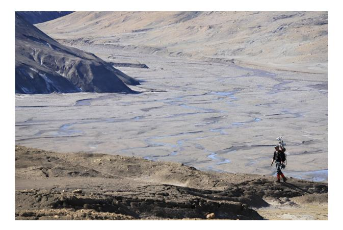
Antero Kukko collecting topographic data using the AkhkaR4DW backpack mobile laser scanning system which Dr. Kukko designed and built. Credit: Shawn Chartrand
