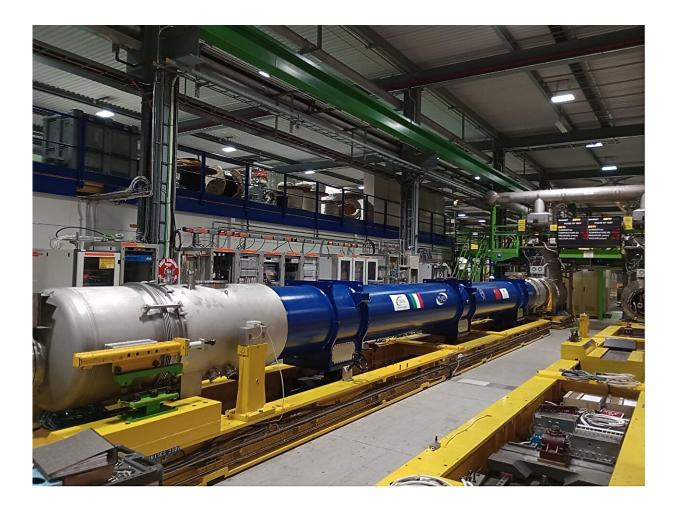
The longest HL-LHC cold mass, integrating magnets from Italy, China and CERN, on the test bench. Credit: CERN
