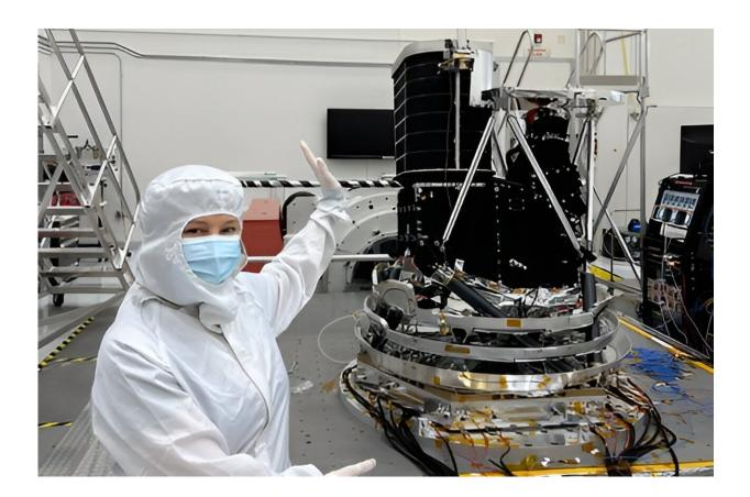
JPL Director Laurie Leshin poses with SPHEREx at JPL. The instrument is mounted to a vibration table for simulating shaking during launch. Credit: NASA/JPL-Caltech
