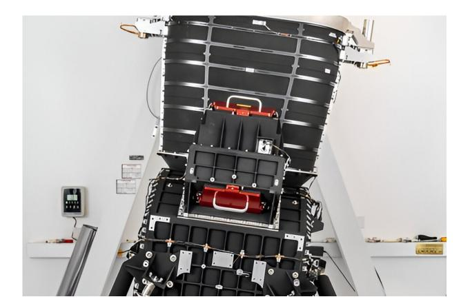
The telescope is tilted to allow SPHEREx to map the entire sky. SPHEREx must carry out its observations without letting sunlight into the thermal system, which means the sun must always be more than 90 degrees off the central axis. If the telescope were pointed straight up, this constraint would leave two holes in the
