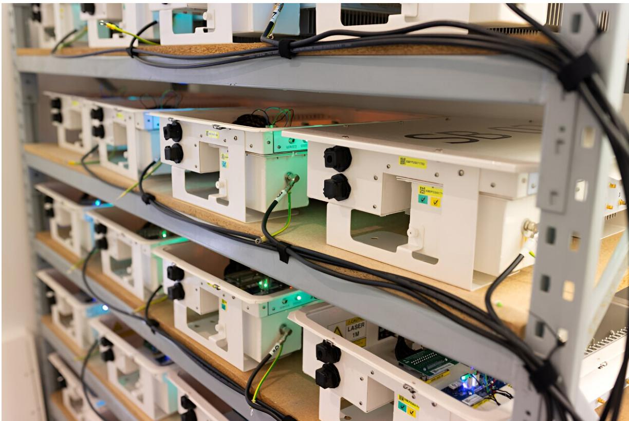
Twenty-four prototype PaSD SMART boxes ready to be installed at the SKA site. Credit: ICRAR
