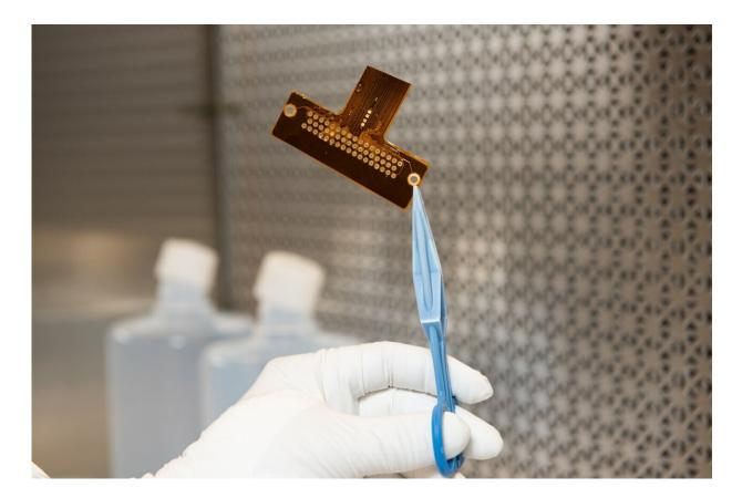
Close up of an ultra-low radiation electronic cable with dozens of conductive circuitry pathways to monitor sensitive physics experiments. This sample cable allows the research team to assess radiopurity after production and cleaning. Credit: Andrea Starr | Pacific Northwest National Laboratory
