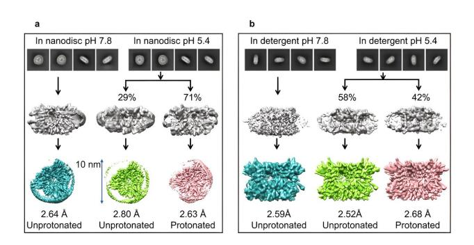
Cryo-EM structures for LHCII in nanodisc and in detergent solution at pH 7.8 and 5.4. Credit: Institute of Physics
