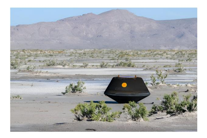
The sample return capsule from NASA's OSIRIS-REx mission, shown blackened from its reentry through Earth's atmosphere, parachuted safely down to the Utah desert on Sunday, Sept. 24, 2023. The capsule contains about 250 grams of regolith, or soil, from the near-Earth asteroid Bennu, which the mission's spacecraft collected in October 2020. The sample's primitive contents could give clues to the first materials that shaped the early solar system. Credit: NASA/Keegan Barber
