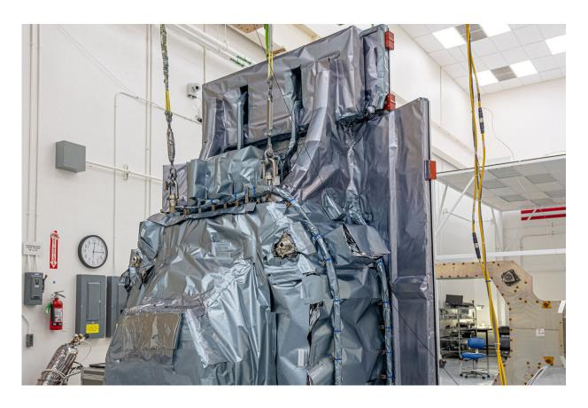
A close-up view of Roman's Wide Field Instrument, currently wrapped in a multilayer insulation for testing. Credit: Ball Aerospace
