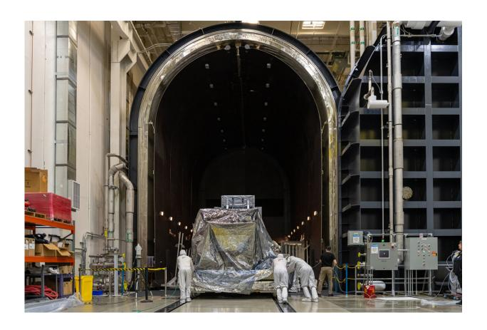
After completing final integration, Ball Aerospace technicians transport the Nancy Grace Roman Space Telescope's Wide Field Instrument (WFI) into Ball's largest thermal vacuum chamber to begin environmental testing at a Ball facility in Boulder, Colorado. Credit: Ball Aerospace
