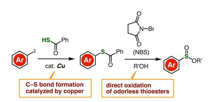
Schematic of the proposed two-step synthesis route to easily produce a wide variety of sulfinate esters. The use of aryl iodides, which are readily available, is a remarkable advantage. Credit: Suguru Yoshida from Tokyo University of Science
