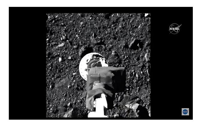
This image from a NASA video shows the robot arm of the Osiris-Rex probe collecting samples from the asteroid Bennu on October 21, 2020.
