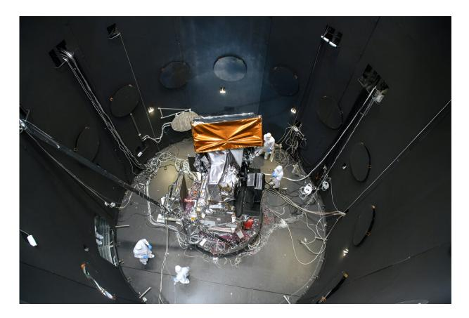
An overview of the PACE satellite entering a thermal vacuum chamber. Before the doors closed, the whole observatory was run through additional testing. Credit: NASA's Goddard Space Flight Center/Denny Henry
