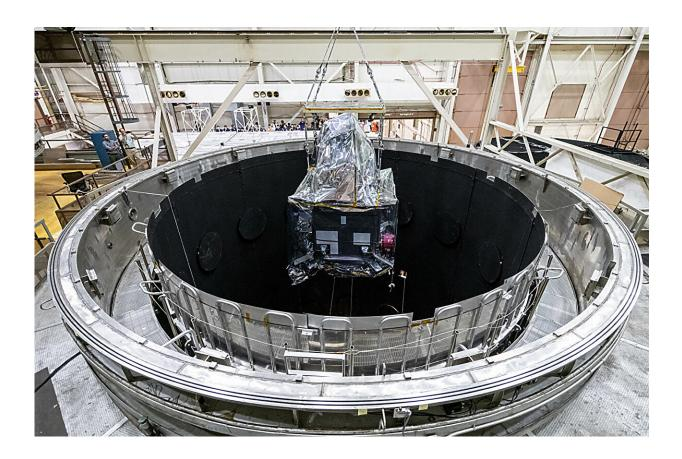
The PACE observatory enters a thermal vacuum chamber at NASA's Goddard Space Flight Center in Greenbelt, Md. It stayed in the chamber for 33 days of testing. Credit: NASA's Goddard Space Flight Center/Denny Henry
