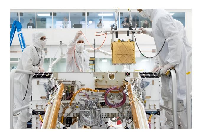
MOXIE (Mars Oxygen In-situ Resource Utilization Experiment) is lowered into the chassis of NASA's Perseverance in 2019. During the mission, MOXIE extracted oxygen from the Martian atmosphere 16 times, testing a way that future astronauts could make rocket propellant that would launch them back to Earth. Credit: NASA/JPL-Caltech
