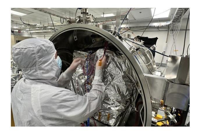
An engineer prepares the imaging spectrometer instrument for testing in a
