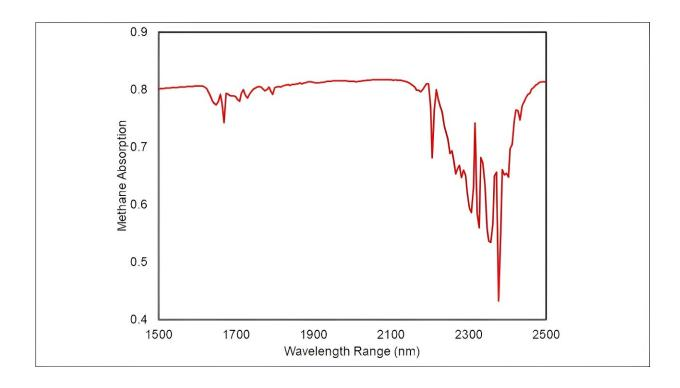
This spectral "fingerprint" of methane was produced from data taken during a test of the imaging spectrometer at JPL. Part of an effort led by the nonprofit Carbon Mapper, the state-of-the-art instrument measures hundreds of wavelengths of light reflected by Earth's surface and absorbed by gases in the atmosphere. Credit: NASA/JPL-Caltech
