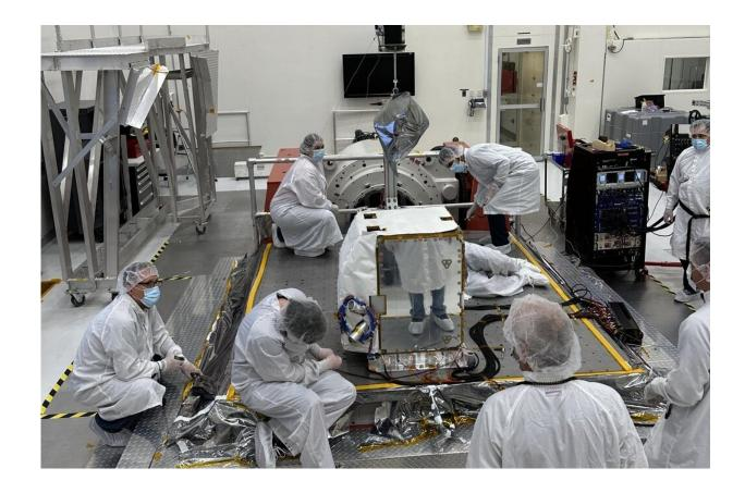
Engineers prepare the imaging spectrometer – part of an effort led by the nonprofit Carbon Mapper to monitor greenhouse gas emissions – for vibration testing at JPL. Credit: NASA/JPL-Caltech
