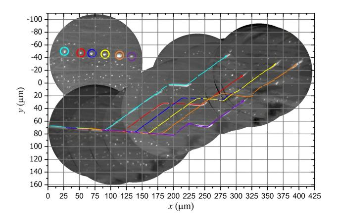
Snapshots from a PEEM movie (field of view 150 micron, 4.9 eV photons) of Ge-Pt droplets. The straight-line segments illustrate the evolution of the positions of the center of gravity, coordinates (x, y) in microns, of the eutectic droplets marked by colored circles in the image in the top-left. The white points are smaller droplets (diameter Physical Review Letters (2023). DOI: 10.1103/PhysRevLett.131.106201
