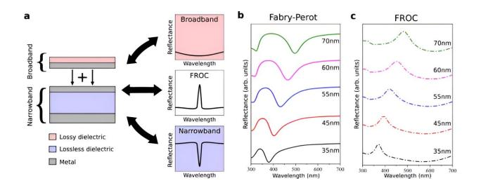
a A FROC consists of two coupled light absorbers; a broadband absorber and a narrowband (Fabry-Perot, FP) absorber. A FROC exhibits a reflection peak at the FP cavity resonance. b The measured reflection from a FP cavity with different dielectric thickness. c The measured reflection from the same FP cavities shown in (b) after depositing a 15 nm Ge film to create a FROC. The incidence angle in (b) and (c) is 15°. Credit: *Nature Communications* (2023). DOI: 10.1038/s41467-023-39602-2
