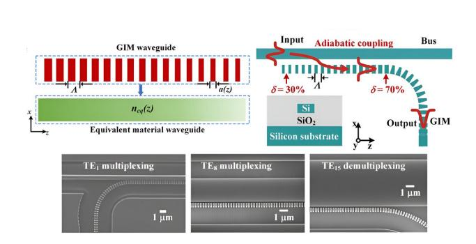
Metamaterials enable specific light propagation modes using a multimode waveguide. (Left) Conceptual illustration of a 1D gradient-index metamaterial (GIM) structure with refractive index continuously varying along the direction of light propagation. (Right) GIM-based coupler for a 16-channel MDM system; (bottom) SEM images of coupling regions. Credit: He et al., doi 10.1117/1.AP.5.5.056008.
