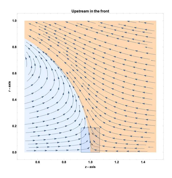
The streamline of Hill's spherical vortex in the moving frame (Upstream in the front). Credit: *Communications on Pure and Applied Mathematics* (2023). DOI: 10.1002/cpa.22134
