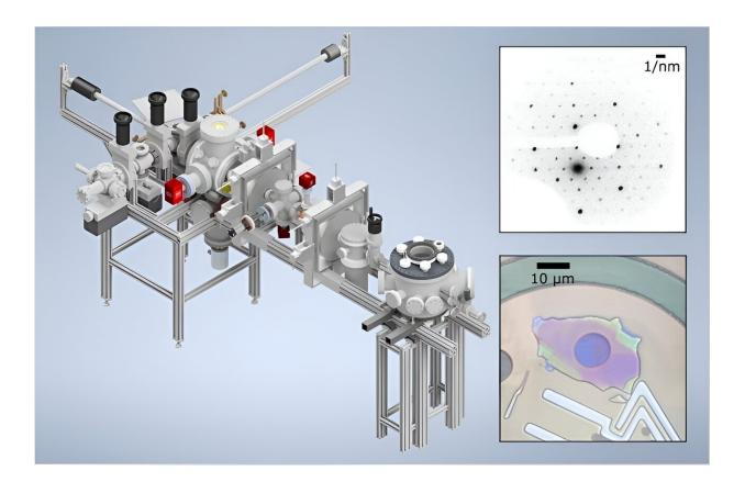
The new ultrafast electron probe apparatus is 3 meters long (left). The diffraction pattern (top right) encodes detailed information on the positions of the atoms within a small sample flake (bottom right). Credit: Cornell University
