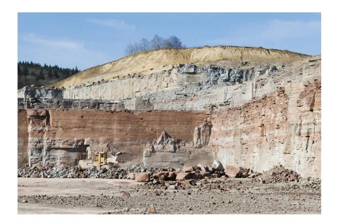
When limestone is quarried and used as a raw material in the production of cement, large amounts of carbon dioxide are released. The industry is working with researchers to find more environmentally friendly alternatives. Credit: Heidelberg Materials
