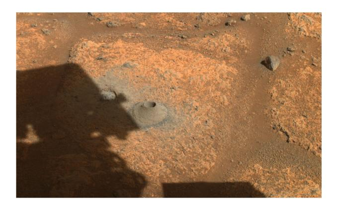
This image taken by NASA's Perseverance rover on Aug. 6, 2021, shows the hole drilled in a Martian rock in preparation for the rover's first attempt to collect a sample. It was taken by one of the rover's hazard cameras in what the rover's science team has nicknamed a "paver rock" in the "Crater Floor Fractured Rough" area of Jezero Crater. Credit: NASA/JPL-Caltech
