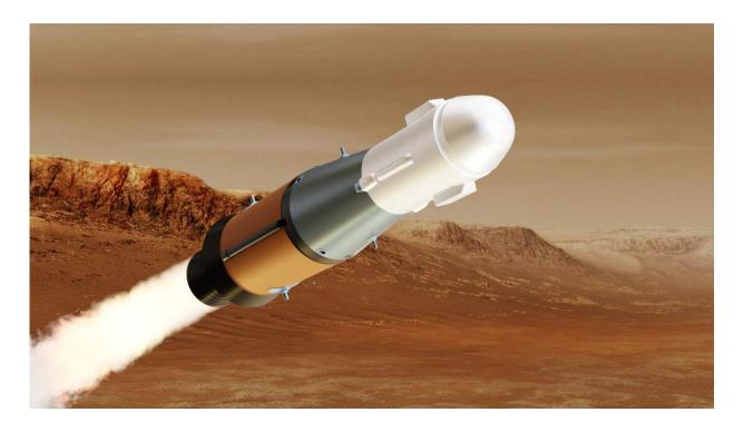
This illustration shows NASA's Mars Ascent Vehicle (MAV) in powered flight. The MAV will carry tubes containing Martian rock and soil samples into orbit around Mars, where ESA's Earth Return Orbiter spacecraft will enclose them in a highly secure containment capsule and deliver them to Earth. Credit: NASA
