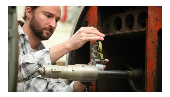
A scale model of the Mars Ascent Vehicle is loaded by Wind Tunnel Test Engineer Sam Schmitz into the trisonic wind tunnel at NASA's Marshall Space Flight Center for testing. The 14-by-14-inch tunnel has been used to test launch vehicle configurations for Artemis, Redstone, Jupiter-C, Saturn, and more. Credit: NASA/Jonathan Deal
