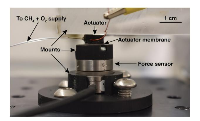
Blocked force testing configuration. A Nano17 Titanium force sensor was used to collect force data at 20 and 40 kHz sampling rates. Credit: *Science* (2023). DOI: 10.1126/science.adg5067
