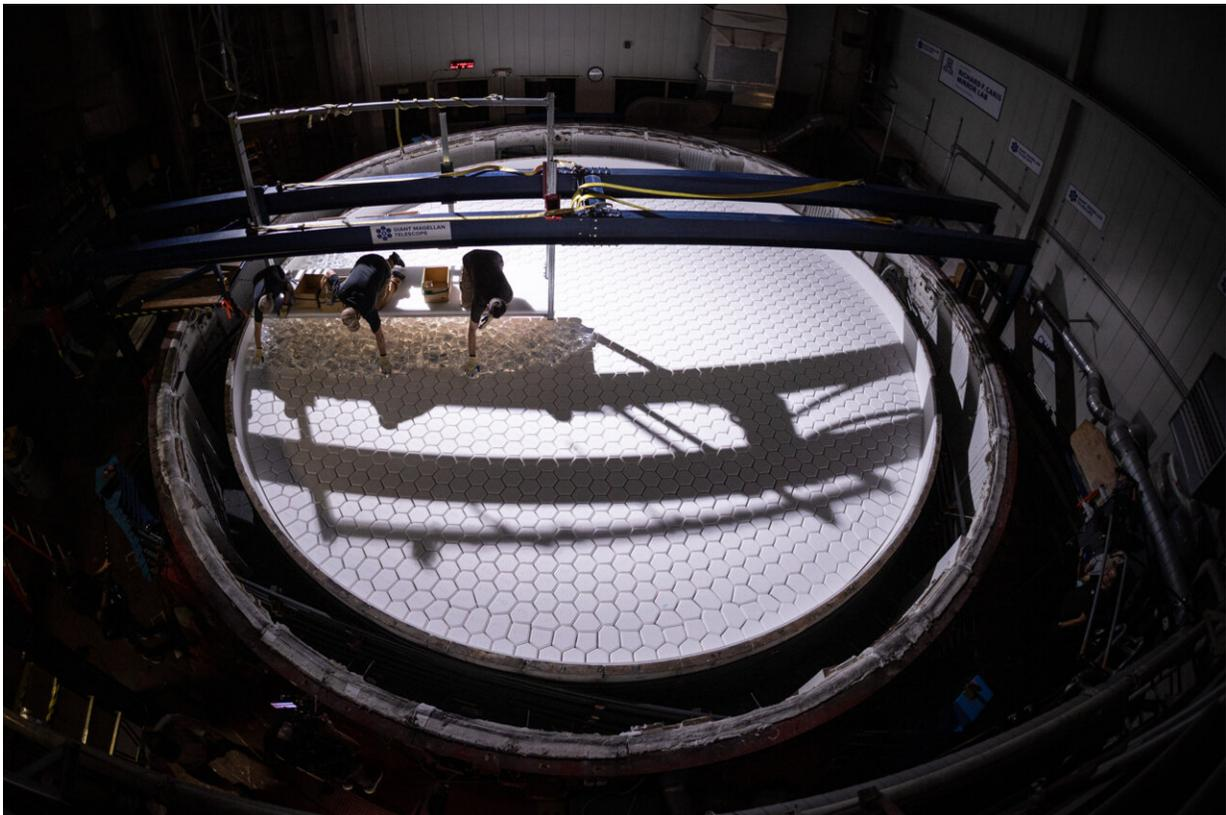
University of Arizona Richard F. Caris Mirror Lab staff members placing chunks of Ohara E6 low expansion glass into a mold for casting the Giant Magellan Telescope's seventh primary mirror segment, September 2023. Credit: Damien Jemison, Giant Magellan Telescope – GMTO Corporation
