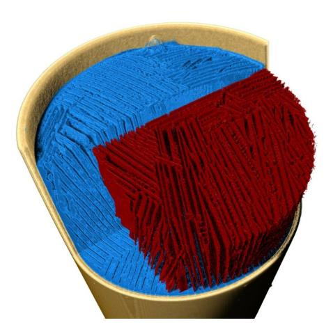
A 3D-rendered tomogram shows a cross-section through the solidified sample in which two phases have separated: the pure ice crystal phase in blue and the sugar phase in red. The lamellar structure formed by the snowflake-like ice crystals is clearly visible. Credit: HZB/PSI
