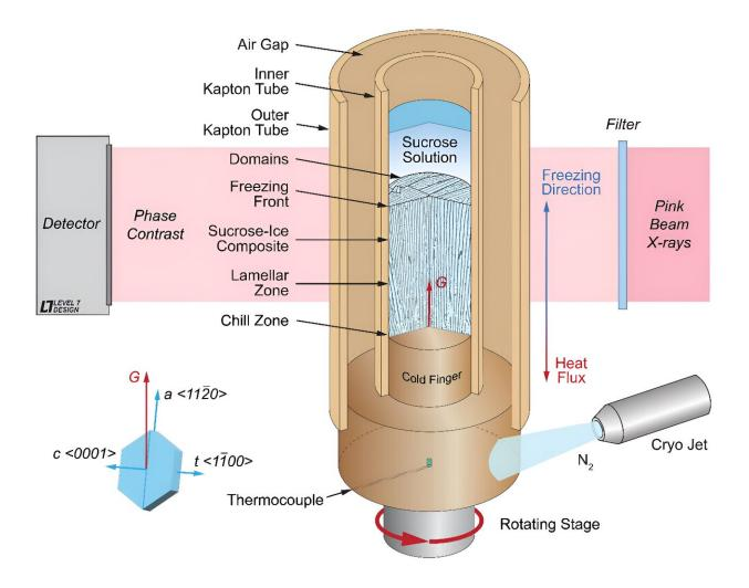
The mold bottom is cooled on the turntable with liquid nitrogen and simultaneously analyzed with X-rays. Ice crystals nucleate on the "cold finger" and grow in the direction of the temperature gradient. During solidification,
