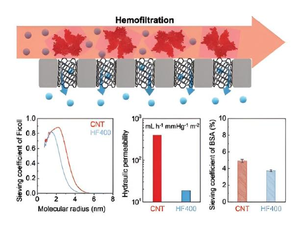
Wafer-scale vertically aligned carbon nanotubes (CNT) integrated into a membrane platform comprising sub-5 nm channels/capillaries enable overcoming persistent challenges in hemofiltration/hemodialysis. Compared with conventional membranes, CNT membranes allow for greatly enhanced removal of middle molecules ( $\approx$ 15–60 kDa) while maintaining comparable albumin ( $\approx$ 66 kDa) retention and significantly higher hydraulic permeability (more than an
