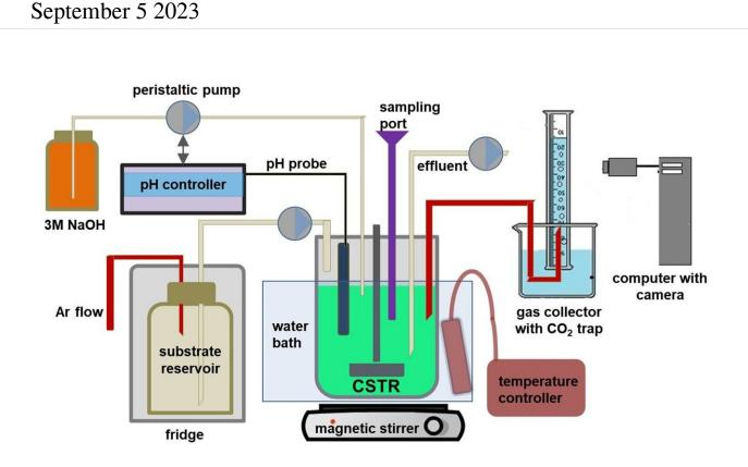
Schematic representation of the experimental set-up. Four identical bioreactors were placed in a single water batch. Credit: *Bioresource Technology* (2022). DOI: 10.1016/j.biortech.2022.127309
