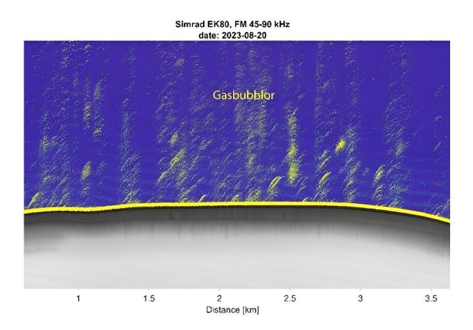
With the help of advanced sonar, the researchers can observe the water column and, in this case, the gas bubbles rising from the ocean floor to the surface. The sonar also penetrates the bottom sediments, which provides important information about the properties of the seabed and, for example, whether there is gas hidden in the sediments. Credit: Christian Stranne
