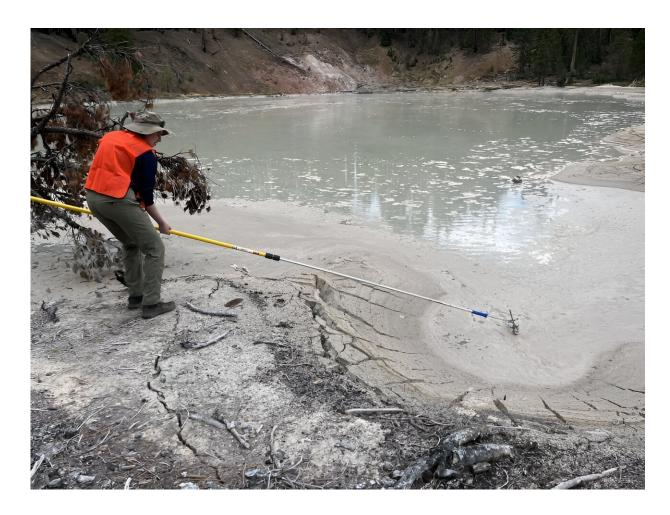
Syracuse University researcher Hannah Rappaport dipping a bottle into a hot lake to obtain a sample. Due to the high temperature of the water and unstable ground, researchers must remain at a safe distance away when collecting samples. Credit: Syracuse University
