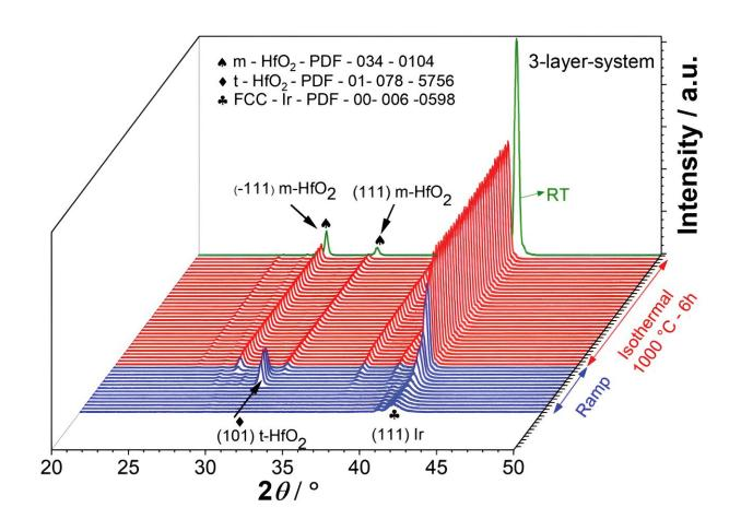
In situ XRD diffractograms of a 3-layer system from room temperature up to  $1,000^{\circ}$ C represented in blue. Diffractograms in red represent isothermal annealing at  $1,000^{\circ}$ C for 6h at  $2 \times 10^{-6}$ . The last scan in green is measured at room temperature at the end of the annealing experiment. Credit: *Advanced Materials* (2023). DOI: 10.1002/adma.202305922
