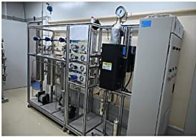
EMF assisted H-B equipment with production rate of 1.25 kg/h-NH 3
