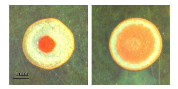
As paint drops dry, they can look like a "fried egg" (left image, scale bar is one millimeter) or develop a more even pigment distribution (right image). Credit: Adapted from *Langmuir* 2023, DOI: 10.1021/acs.langmuir.3c01605
