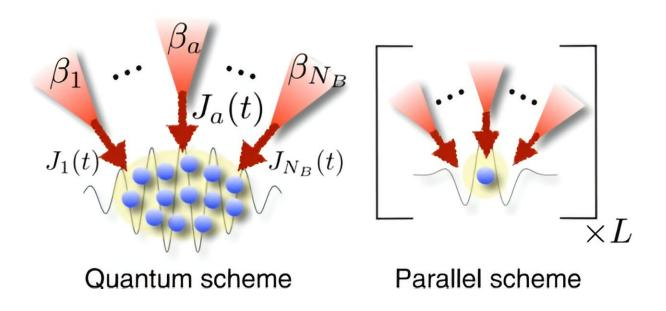
Schematic for a quantum scheme for heat current generation realized in a system composed of *L* particles surrounded by  $N_B$  baths. For a parallel scheme, the *L* particles are used in parallel. Credit: *Physical Review Letters* (2023). DOI: 10.1103/PhysRevLett.131.090401
