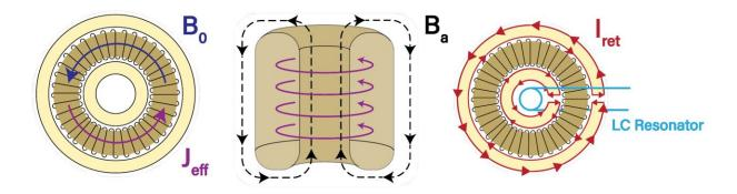
Figure 2: A schematic representation of DMRadio-50L. The magnetic field we apply  $(B_0)$  will interact with the dark matter axions to produce the axion induced current  $(J_{eff})$ . This in turn will induce a flux in the center of the toroid and then the currents that flow in response to that  $(I_{ret})$  are resonantly enhanced and measured. Credit: DMRadio Collaboration
