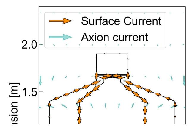
Figure 3: A cross-section of the DMRadio-m<sup>3</sup> resonator. The magnetic field, and hence the axion current, flows along the teal lines. That in turn induces a current to flow on the surface of the resonator—that is the current that our experiment will try to measure. Credit: Electromagnetic modeling and science reach of DMRadio-m<sup>3</sup>
